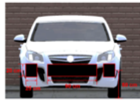
Fig. 2. Signaling interface consisting of three displays at the front of the car. The side displays have been rotated by 43° for better adjustment to the vehicle front.
